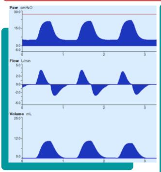
Most ventilator screens that you will see will show the three waveform graphics shown here; pressure, flow and volume. All with time as the x-axis.
