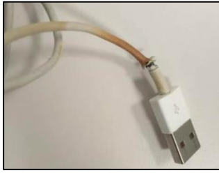
Damaged charger cable / signs of overheating
