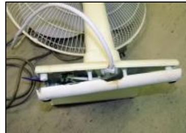
Loose / damaged equipment covers
