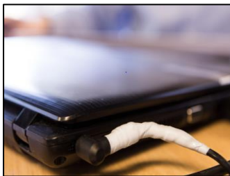
Damaged cable repaired with tape
