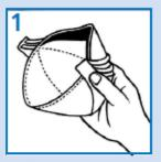
Hold the respirator in one hand and separate the edges to fully open it with the other hand. Bend the nose wire (where present) at the top of the respirator to form a gentle curve.
