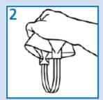
Turn the respirator upside down to expose the two headbands, and then separate them using your index finger and thumb. Hold the headbands with your index finger and thumb and cup the respirator under your chin.
