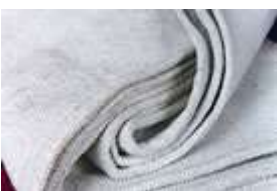
Fig 1: Asbestos fire blanket.
