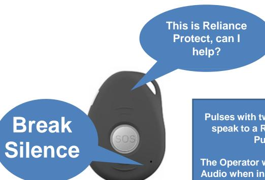
Pulses with two way audio enabled allow the user to speak to a Reliance Protect Operator through the Pulse when in SOS activation.
