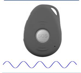
Vibration every 30 seconds (You can stop the vibrations by using the USB cable to charge if required) Battery 10% or less > (at least 1 to 2 hours battery life remaining)
