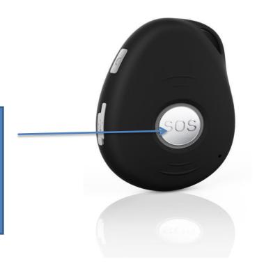
Once connected, the Pulse will vibrate twice every ten seconds. This is your reassurance that you are connected to Reliance Protect's Alarm Receiving Centre (ARC).
