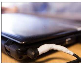
Damaged cable repaired with tape
