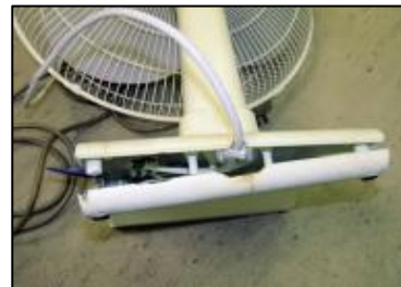
Loose / damaged equipment covers
