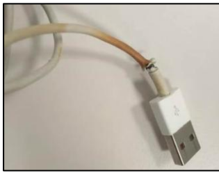
Damaged charger cable / signs of overheating
